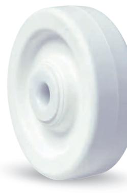
Hamilton Aqualite® Wheels are of the genre loosely referred to in the industry as "polyolefin" or "polypropylene," but unlike most competitive designs they have heavily-sectioned hubs and rims to withstand the rigors of industrial service. They are injection molded from blended polymers that provide an impact-resistant wheel (75 Durometer on Shore D) impervious to water, brine, gasoline and oil, and most
