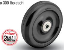
This hard tread polyolefin wheel is light weight, offers non-marking floor protection, and resists hard impacts. Very light in weight, yet the impact strength for this wheel is far superior to hard rubber wheels. It offers superior resistance to most oils, chemicals, grease, solvents and acids. Fit for light and medium duty applications. The standard color is black.
