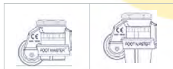
One moving and one set / a caster combined with a leveling
